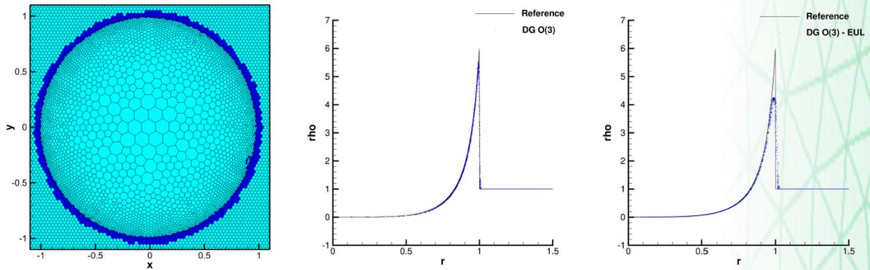
Figure 5: Sedov explosion problem solved with our third order ALE-DG scheme. The topology changes maintain a high quality mesh and the Lagrangian framework (middle) allows to obtain a scatter profile perfectly in agreement with the reference solution and much better than what obtainable with an Eulerian scheme (right) of the same order. Note that our a posteriori FV limiter activates exactly only at the shock location (blue cells in the left panel).
