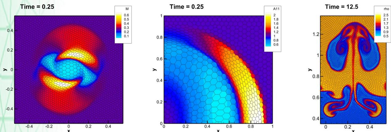
Figure 7: MHD rotor problem, explosion problem in an elastic solid, Rayleigh-Taylor instabilities.
