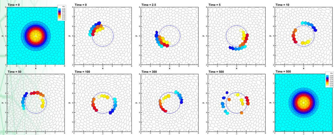
Figure 4: Stationary rotating vortex solved with our fourth order ALE-DG scheme. Density contours at  $t = 0$  and  $t = 500$  and position of a bunch of highlighted elements at different times. Note that the solution is well preserved for more than fifty complete loops and generator trajectories are perfectly circular!
